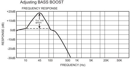
The BASS BOOST control raises the amplifier output up to 18dB at frequencies tightly centered around 45Hz. This "bump" can have a dramatic affect on the bass system's apparent volume. Use caution(!) When adjusting this control as serious subwoofer damage may result from overpowering or overexcursion.
